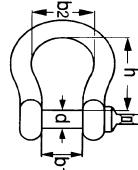
**D SHACKLES WITH COUNTERSUNK HEAD PIN FOR USE WITH SCREW DRIVER OR BIT KEY ACC. TO YOUR CHOISE.**
